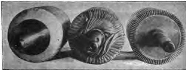
FIG. 18.—A TOOTHED-CORE ARMATURE SHOWING THE STAGES OF WINDING.
